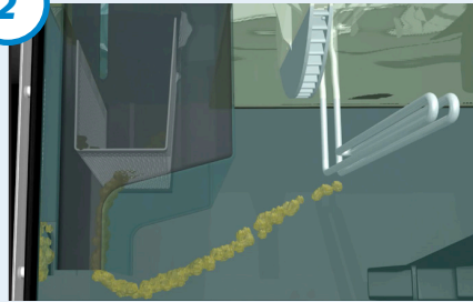
Grease Flows through Stainer Basket into Tank
